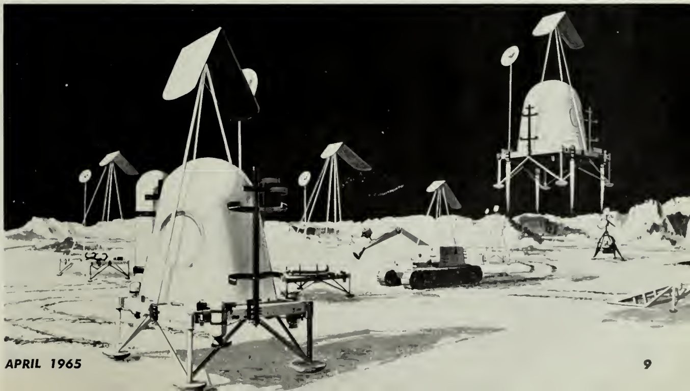
One concept on moon landing and return is shown here. Tracked transport fuels return module (foreground) with rocket motors. Manned module (rt.) lands from orbiting Apollo when return vehicle is ready. Operation is monitored from Earth by TV surveyor at right rear.
